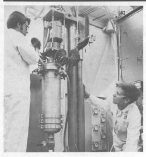
THIS BENCH-SCALE REACTOR, once located in Bldg. 894, was a workhorse for coal-liquefaction lab experiments during the mid- and late 70s. Here, Jim Lyons (now 7471) pours coal slurry into reactor's preheater before a test. Dave Hawn (also 7471) looks on. The reactor has since been dismantled and replaced.
